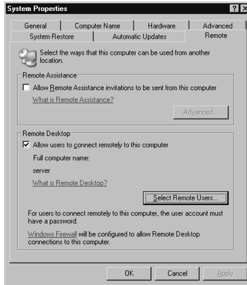
Figure 2.38 Enabling Windows Terminal Services
